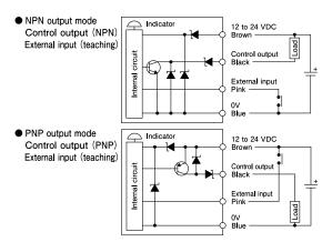
\*\* When not using the external input, connect the external input cable (pink) to 12 to 24 VDC in NPN mode and to 0V in PNP mode.
